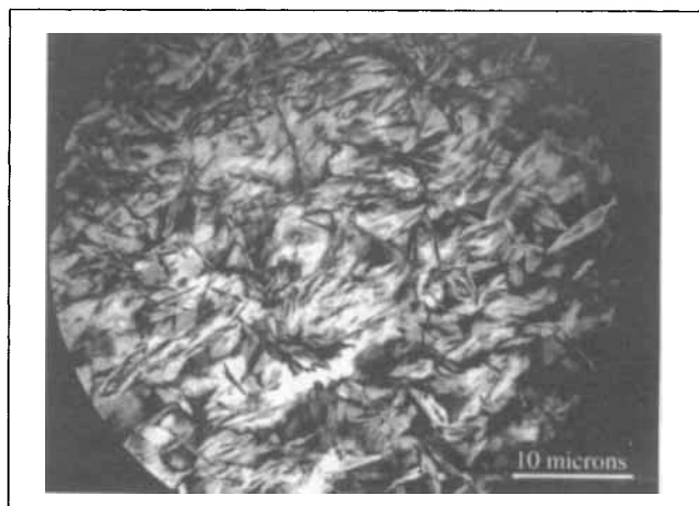
Figure 2. Microscopic image of the incipient gel layer deposit in a flow cell under a laminar flow.
